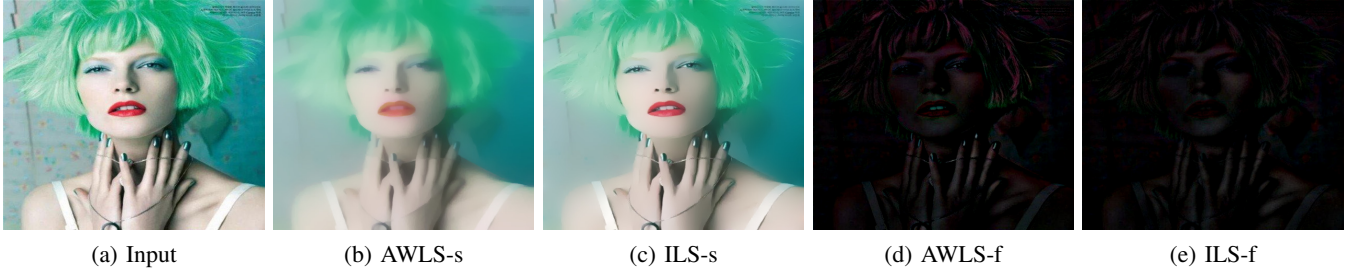
Fig. 5. Image smoothing comparison. (a) Input image. (b, d) Structure and texture layers extracted by AWLS filter, respectively. (c, e) Structure and texture layers extracted by ILS filter, respectively.
